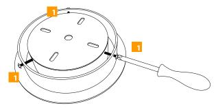
Loosen strain relief screw releasing the rubber strain relief bushing.
